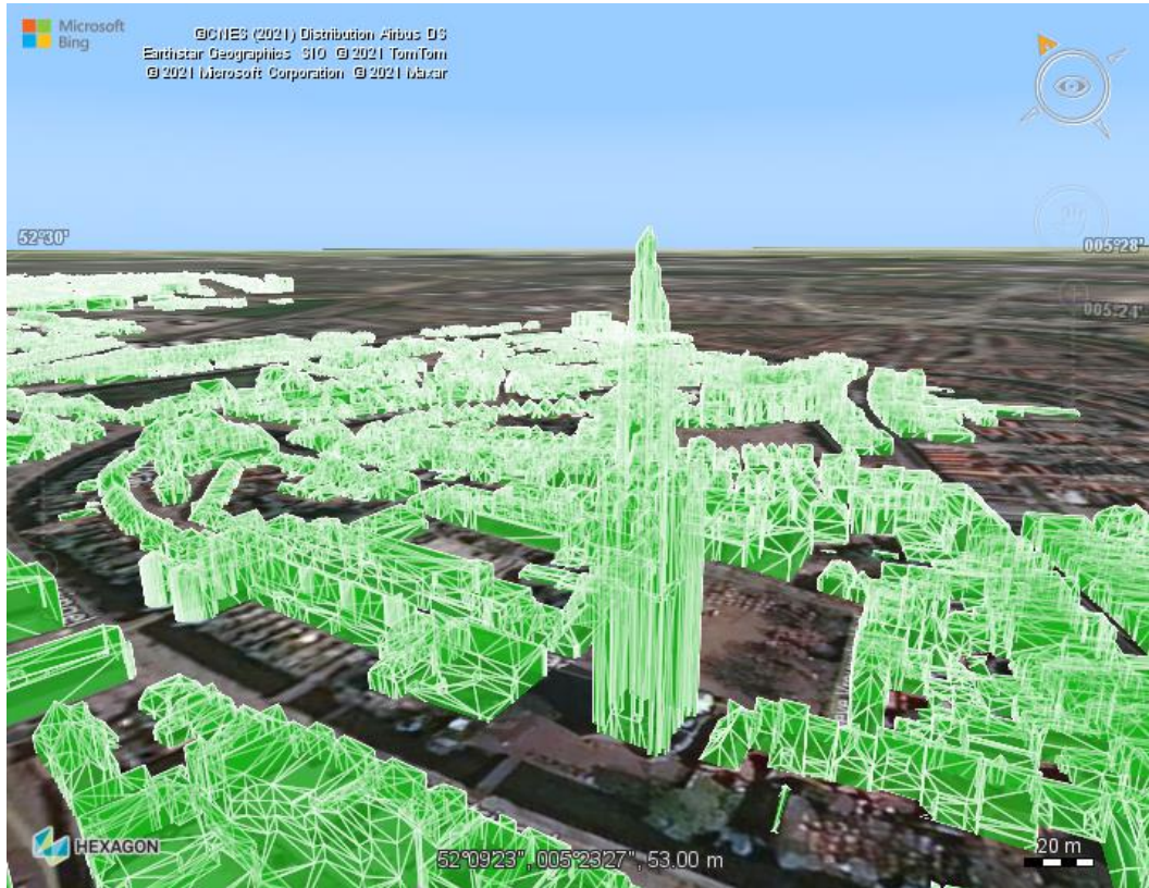
Figure 7: One of the landmarks used for the NAP vertical datum is the church tower in Amersfoort (building data by 3dbag.nl).
