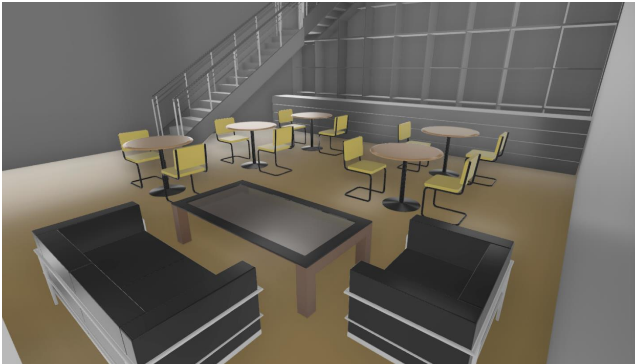
Figure 3: The visualization of a Revit file , after conversion to OGC 3D Tiles
