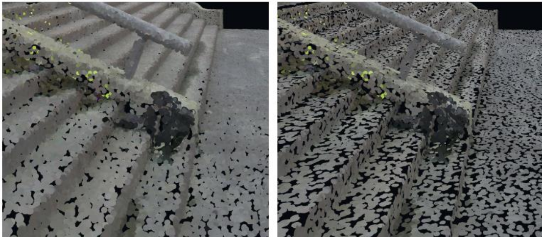
Figure 6: The picture on the left shows a point cloud visualized without considering the normal orientation. The picture on the right shows the result with normal orientation.
