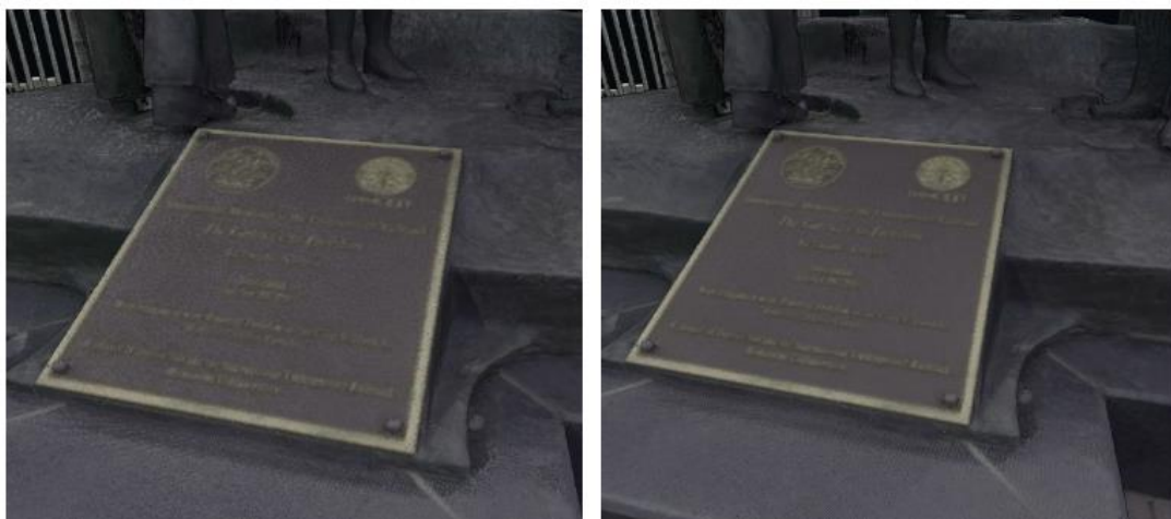
Figure 7: The picture on the left shows a point cloud without blending. The picture on the right shows a point cloud with blending enabled, which improves the readability of the text.
