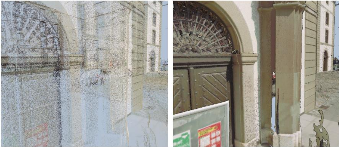
Figure 5: The picture on the left shows an unclear, sparse point cloud. The picture on the right shows this point cloud displayed with high visual quality.
